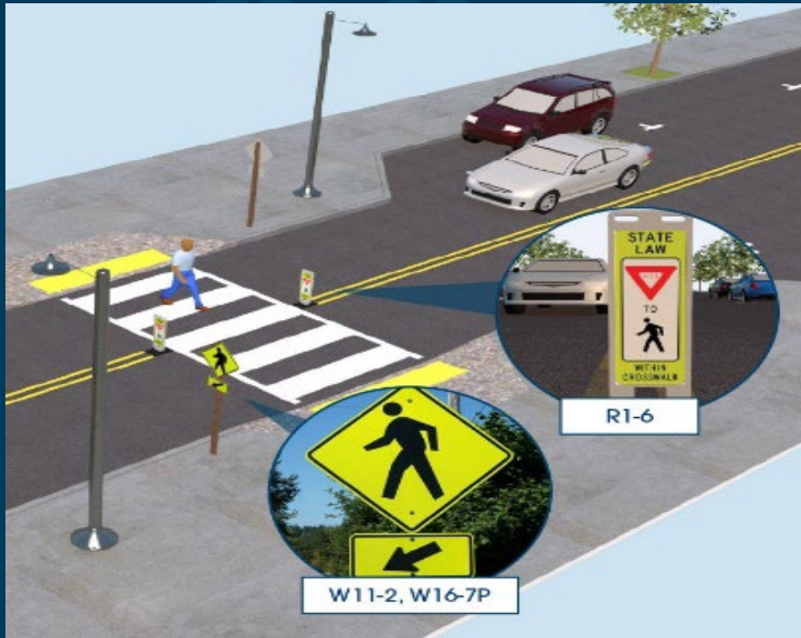
High Visibility Crosswalk Markings (HVCM)
