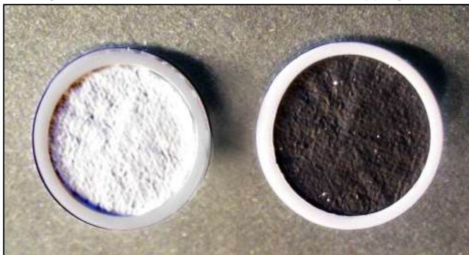
Figure 15: Air Monitor Filter Before and After Trapping PM 2.5
