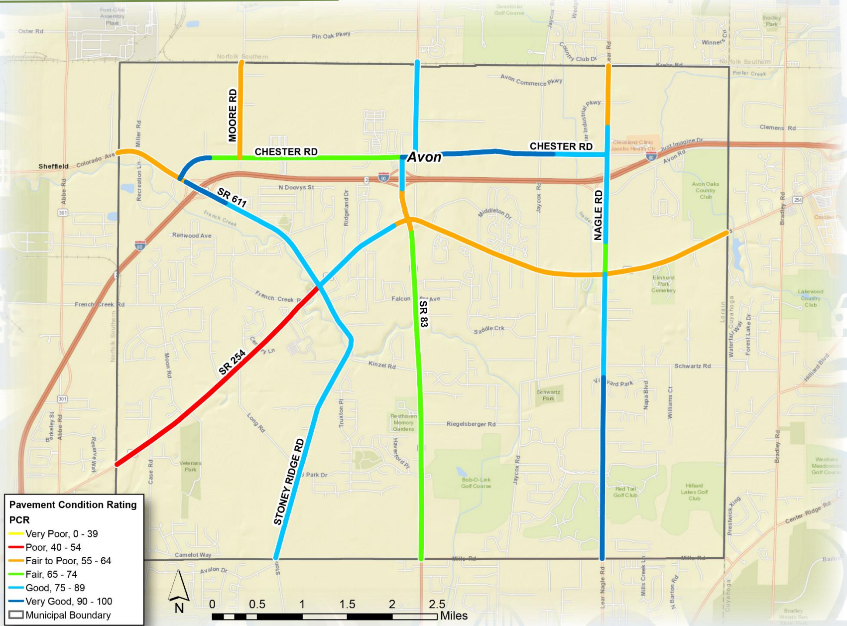
Map 2: 2020 City of Avon Pavement Condition
