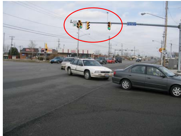
Residual westbound traffic on US20 turning left onto SR306 southbound trapped within the intersection during the green interval for east-west traffic movements due to congestion on the southern leg of SR306
